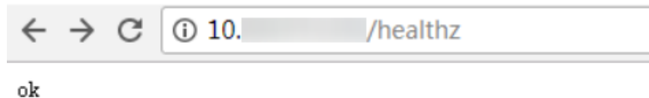
Figure 10-22 Accessing the /healthz interface of defaultbackend
